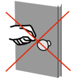
Figure 62 — Examples of door lever handle, pull handle and push plate that may/can be operated easily with a closed fist. Incorrect solution: knob type handle
