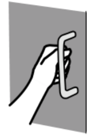
Figure 62 — Examples of door lever handle, pull handle and push plate that may/can be operated easily with a closed fist. Incorrect solution: knob type handle
